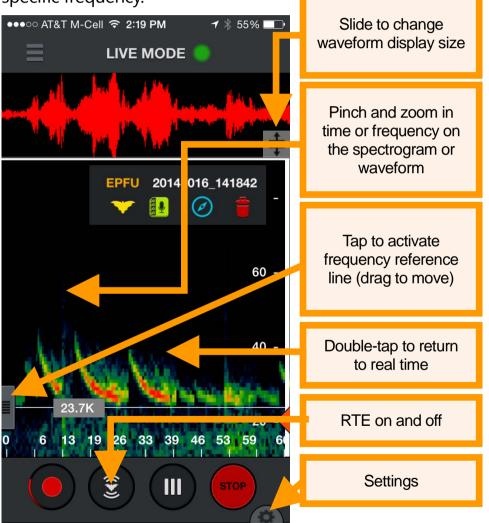
You can also listen to bats using Wildlife Acoustics patented Real Time Expansion (RTE). RTE translates the ultrasonic sounds to a range that is audible to humans by taking tiny snippets of the sound and slowing it down. Since there is quite a bit of space in between bat echolocation calls relative to the length of the call, the space in between is used to play back the slowed down call.
