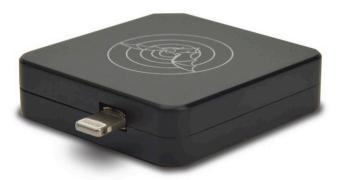
The Echo Meter Touch Ultrasonic Module senses ultrasonic signals up to 125 kHz with an ultrasonic microphone, digitizes the signal, and transmits the ultrasonic data to the iPad or iPhone.
