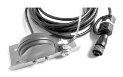
A stainless steel-screen covers the top of the microphone and directs any surges to the bracket and then to the grounding wire. This also provides some protection to the recorder, but the available Song Meter Surge Suppressor should also be used for best protection.
